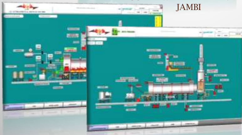
SCADA INCINERATOR CIC
